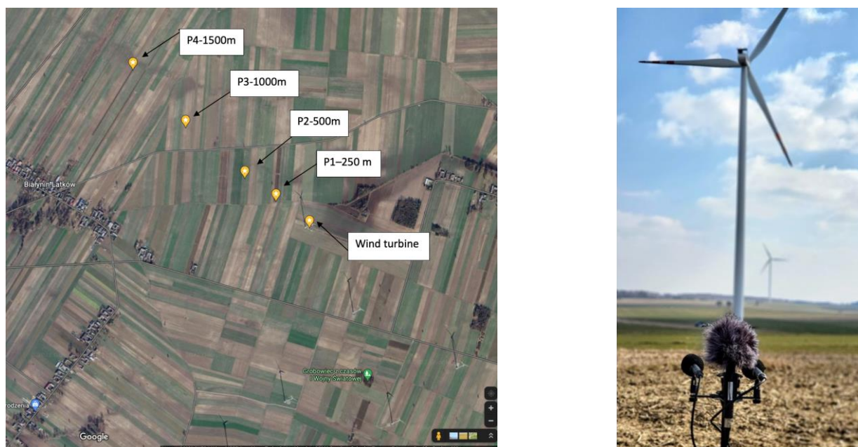
Figure 1. The wind turbine noise measurement and recording points. Satellite photo source: google.maps.com (accessed on 23 June 2022).
