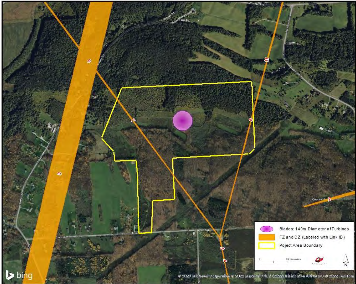
Figure 3: Microwave Paths with Fresnel Zones
