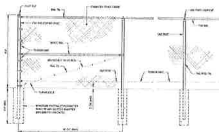
5 CHAIN LINK FENCE DETAIL 1/4" = 1'-0"
